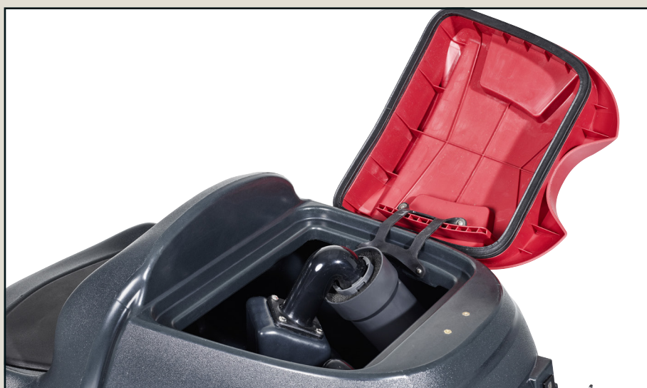
Park the machine leaving the recovery tank cover open
