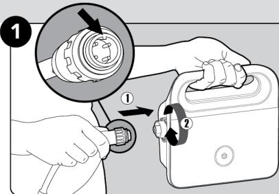
Attach the floating cable to the power supply.
