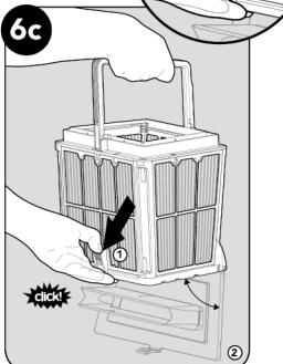
Open the latch to release the bottom lid in order to remove the debris.
