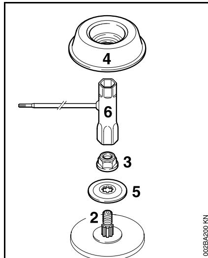
💡 The rider plate (4) is in the parts kit supplied with the machine.
