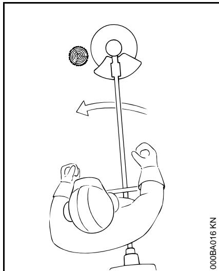
Circular saw blades are suitable for thinning brush and cutting small trees up to a diameter of 4 cm (1 1/2"). Do not attempt to cut trees with larger diameters, since the blade may catch or jerk the trimmer/brushcutter forward. This may cause damage to the blade or loss of control of the power tool and result in serious injury. Use a chain saw for such work.
