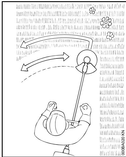
All kinds of grass and weeds can be easily cut with the grass cutting blade. The power tool is swept in an arc similar to a scythe.
