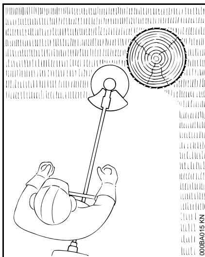
Mowing heads are to be used only on trimmer/brushcutters equipped with a line-limiting blade in the deflector in order to keep the line at the proper length (see "Parts and Controls" chapter in your instruction manual).
