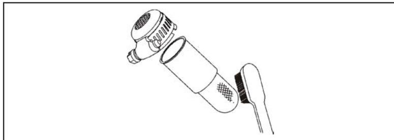
4.Check the muffler gasket; replace if damaged. Reinstall the muffler gasket, the spark arrester, the muffler and the muffler protector in the reverse order of removal.
