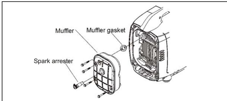
3.Use a brush to remove carbon deposits from the spark arrester screen.
