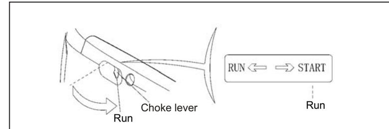
4.Pull the starter grip until resistance is felt, then pull the starter grip briskly toward the arrow as shown below.
