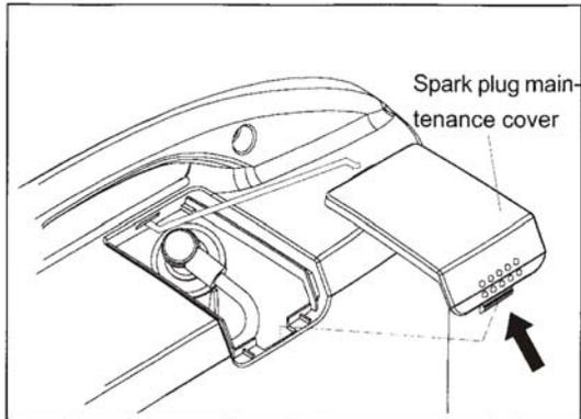
2.Remove the spark plug cap.
