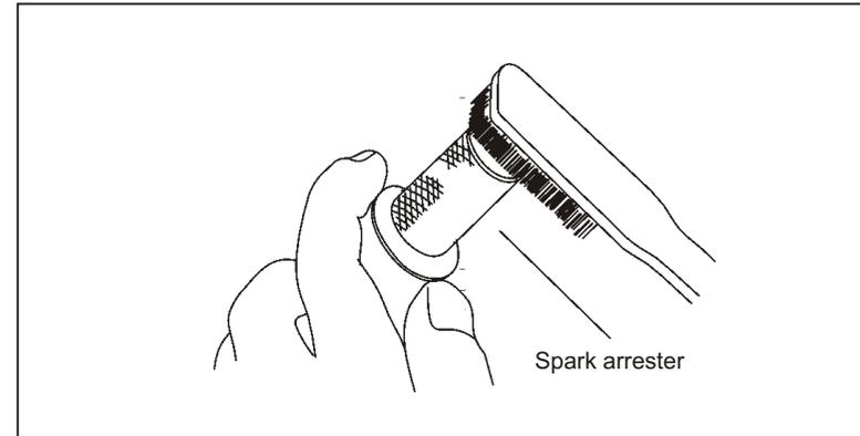
4. Check the muffler gasket; replace if damaged. Reinstall the muffler gasket, the spark arrester, the muffler and the muffler protector in the reverse order of removal.
